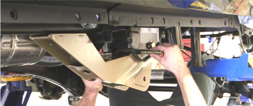
6. Install 3/8"x1.25" hardware into the rear portion of the drop up through the frame rail (nuts on the bottom). Do not tighten at this time.
