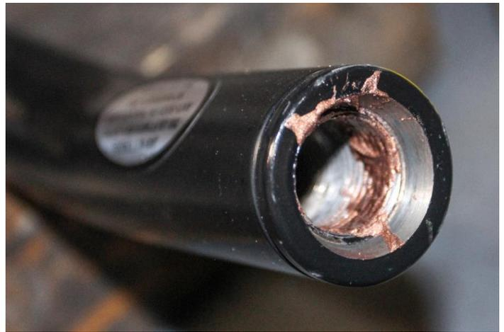
4. Thread the provided jam nut all the way to the end of the shank on the heim-joint so it's tight against the housing. Thread the heim joint 1-2 threads into the track bar. Apply RED LOCTITE to **ALL** the exposed threads of the track bar. These are the threads on which the Tapered-Jam Nut will sit.
