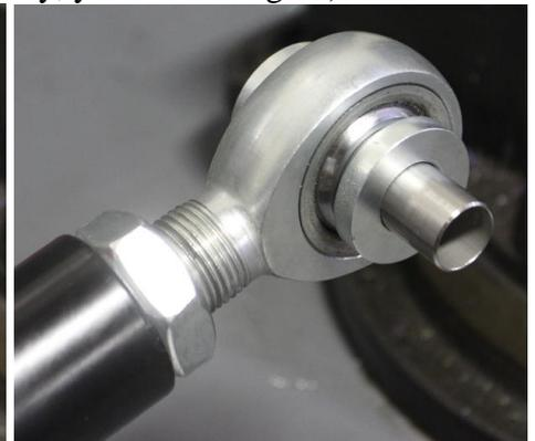
14. Slide the assembled heim joint with misalignment spacers (and reducer where applicable) into the axle pocket and assemble with the factory hardware to be torqued later.
