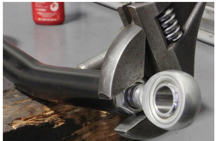
10. Confirm ends remained parallel during torquing.
