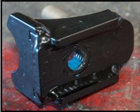
4. Coat the threads of the welded nut in the bracket with medium strength thread locker (we use Blue Loctite) as the stud you're threading in is made of Stainless Steel. Anti-Seize would also work.
