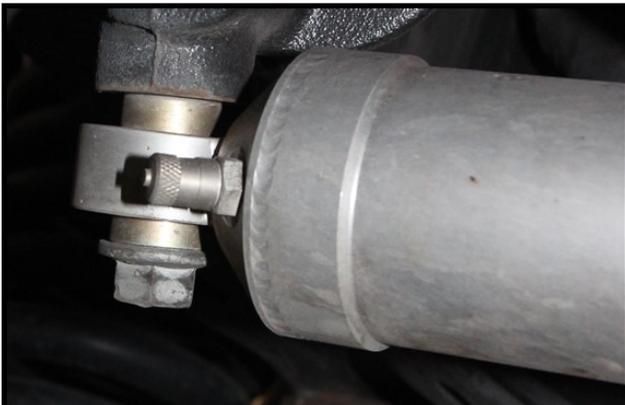
7. Install the body end of the Stainless Shock into the factory frame-side mount using the removed factory bolt and 2 supplied gold spacers; one on each side of the bearing. (pictured)
