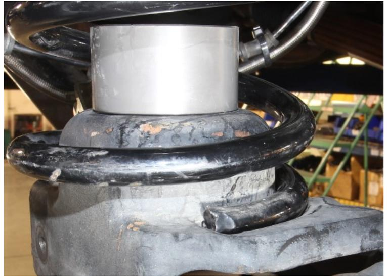
13. Use a Jack under the axle to compress the spring. If this is part of a Carli system, move on to the next instruction; otherwise, reinstall all components removed to install the springs.
