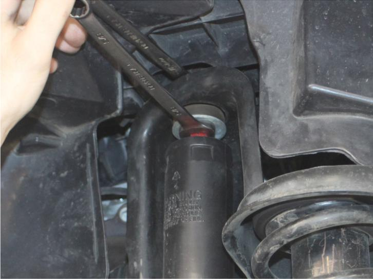
5. Remove the lower shock hardware and remove the shocks from the vehicle.
