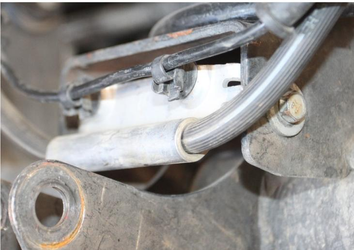
9. Droop the front axle ensuring it's not hanging from the brake lines, axle vent or ABS lines and remove the factory coil springs
