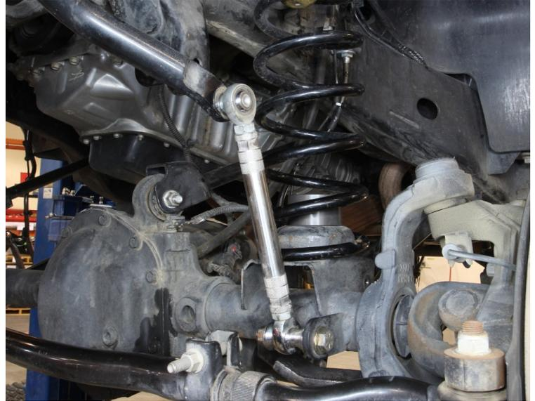
10. From the outside - in, The upper will be arranged: Sway Bar Link, Sway Bar, Flange Nut. **Torque to 75lb.ft.**
