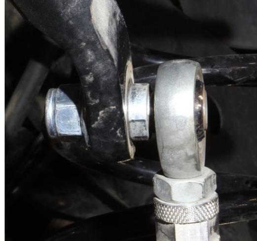
11. From the outside - in, The lower will be arranged: Bolt, Washer, Axle Mount, Large Misalignment Spacer, Sway Bar Link, Small Misalignment Spacer, Flange Nut. **Torque to 75lb.ft.**
