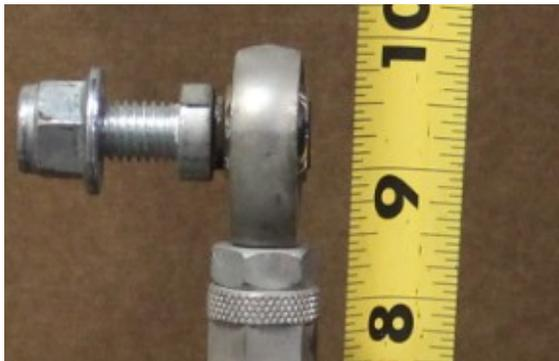
7. With the upper and lower heim joints clocked parallel to each other, tighten the jam nuts to affix the end link's configuration.
