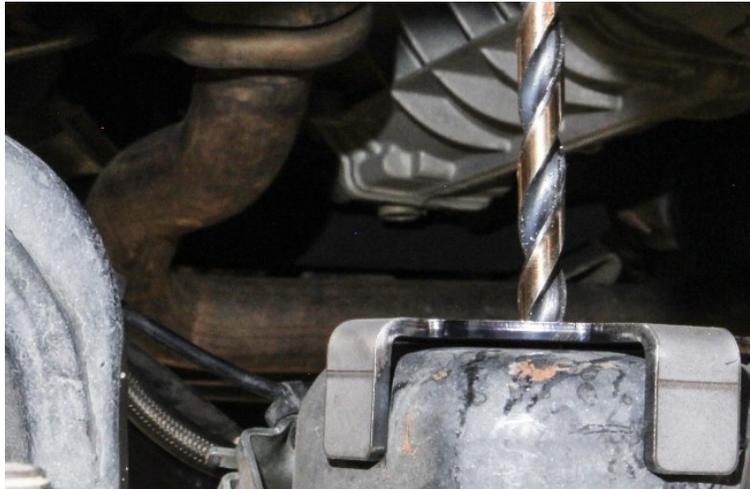
Once drilled, install the bump riser provided with your shock package; **the short meant for the 2.0" IFP and Remote Reservoir will measure 5/8" and the tall meant for the 2.5" Remote Reservoir will measure 1-3/8"**. The Bolt is a 3/8" and the socket used will be a 9/16". Place the bump riser on the drilled surface, insert the bolt into the recess on the bump riser and slide the washer and crimp-lock nut to the underside of the lower spring bucket. **Torque to - 20 lb.ft.**
