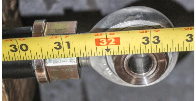
10. Spin the jam nut to the end of the bar and torque using a crow's foot to 200lb.ft. **The joint will not yield until close to 500lb.ft. The more torque, the better. We use a 36" adjustable wrench to take this joint far beyond 200lb.ft.**
