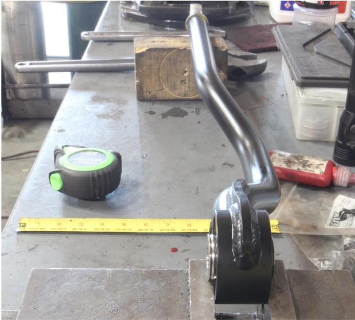
5. Thread the heim joint all the way out until only a couple threads hold it to the bar.
