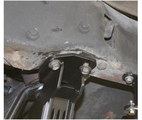
4. Once a few threads are engaged into the frame capture nuts, insert the captured bolt from the back side of the motor crossmember, through the track bar bracket and secure with the factory nut in the recess of the bracket.
