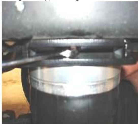
9. Put the 5/8" x 1.25" bolt with washer through outside of frame and thread into the upper air bag bracket. Leave loose.
