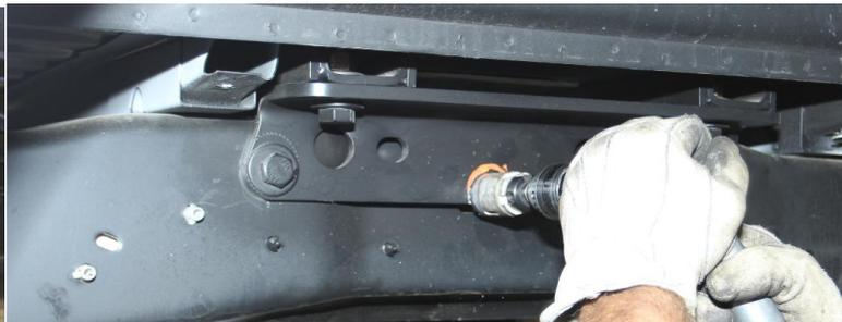
10. Put the 3/8" x 1.25" bolt with washer through the frame, upper air bag bracket and then the brake line bracket. Follow with another washer and c-lock nut.
