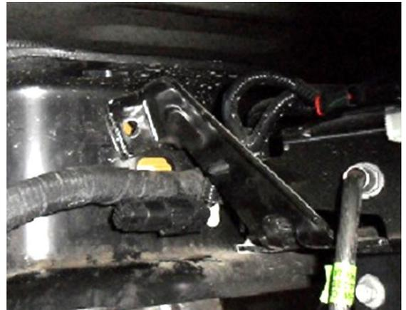
7. Loosen all bolts to the brake line bracket ensuring it can be moved when attempting to fit the upper air bag bracket between the brake line bracket and the frame.
