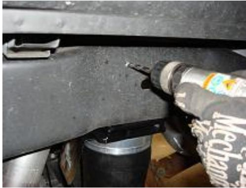
10. Use the supplied 3/8 x 16 x 1 button head bolts through the upper two holes. The button head bolt and washer goes on the outside of the frame. Tighten
