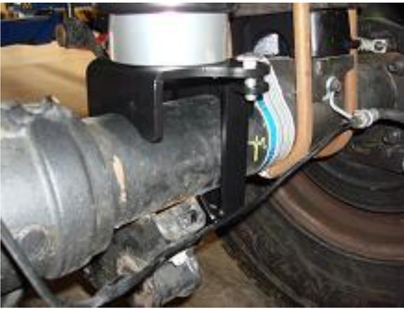
**NOTE:** Tack weld the lower plate to the axle on all 4 corners! This will prevent the lower plates from rotating under extreme torque situations.
