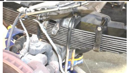
7. Tighten U-Bolts evenly in a cross pattern to 110 lb/ft. These will be re-torqued when the vehicle's weight is on the axle.
