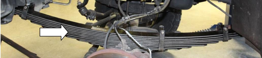
3. Slide the Driver's leaf spring (with the front hanger assembled to it) over the axle from the rear and set the spring on the perch ensuring the center pin lines up with the recessed index.
