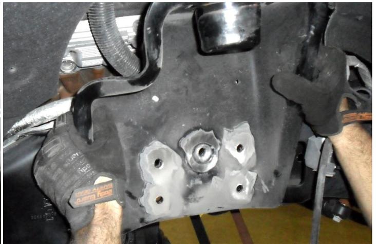
7. Install upper Coil Bucket with supplied 1/2" hardware and torque hardware to 85 lb/ft Torque the bottom bolts first to ensure the bracket is tight to the frame.
