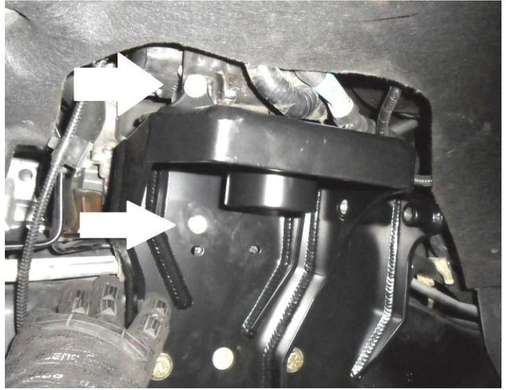
8. Mount previously disconnected wiring loom bracket to new upper coilover mount with supplied 5/16" hardware.
