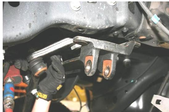
6. Remove bolt on backside of driver's side coil bucket that holds wiring loom bracket.
