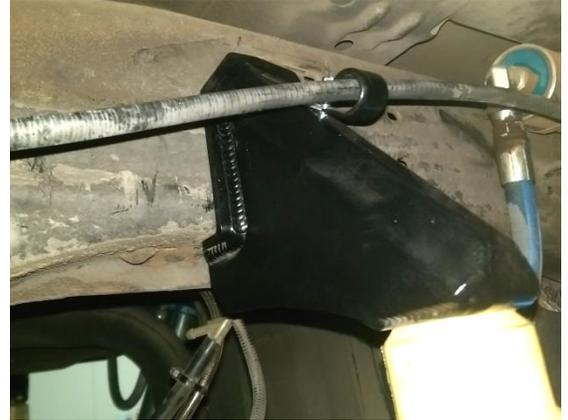
6. Install the Bump stop strike plates into the keyways on the U-Bolt plates on both sides. These plates should fit flush; if they contact a U-Bolt thread, use a cutoff wheel to trim the interfering U-Bolt. Once cleared, assemble plates (sloping to the rear) and install the provided 3/8" hardware and torque to 40lb/ft.
