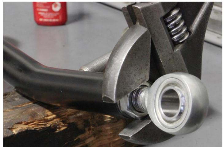
**12. Confirm ends remained parallel during torquing.**
